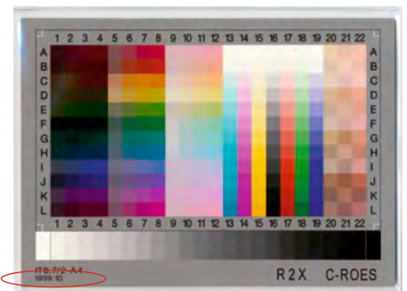
C-ROES target DIN A4, reflective, printed directly on the target - bottom left.
