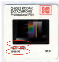
Kodak target 35mm, transparent, reference is date printed directly on the target and also on the slide mount.
