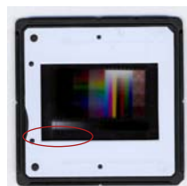
C-ROES target 35mm, transparent, reference is date printed directly on the target
