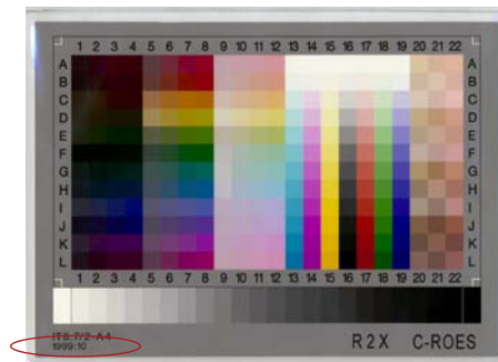
C-ROES target DIN A4, reflective, printed directly on the target - bottom left.
